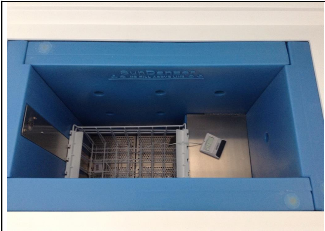
Interior view of Vaccine Fridge indicating heavy insulation and storage racking
